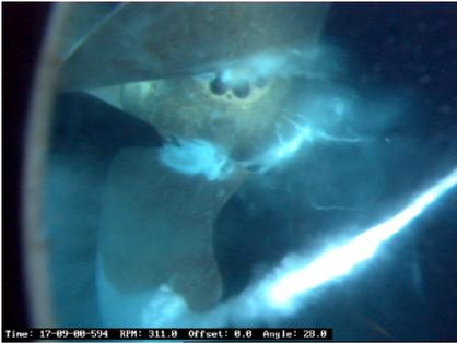
On board propeller cavitation observation
