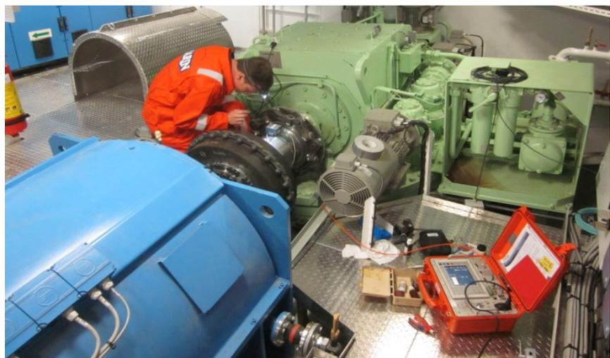
*Shaft power measurement during speed/power trial*
